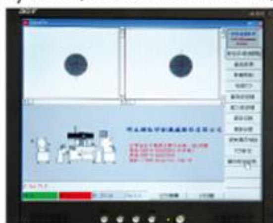
CCD畫面採用TFT-LCD 液晶螢幕 The CCD system utilizes a TFT-LCD monitor.
